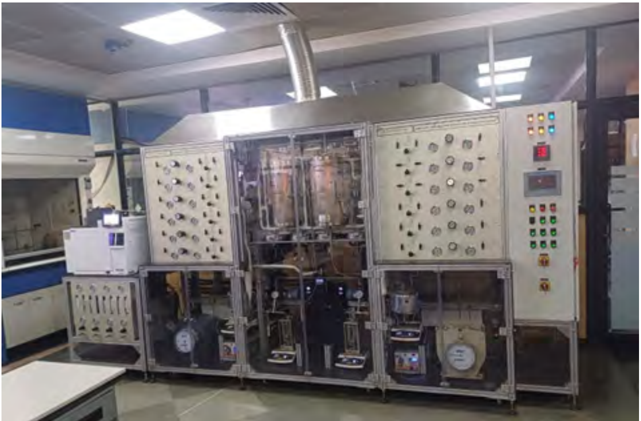
Fixed bed twin reactor setup
